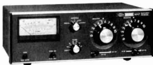
The Drake MN-7. Same features as the Drake MN-2700, but rated at 250 watts. Same width and height, but only 8½" (21.6 cm) in depth, and weighs 10 lbs. (4.55 kg).
