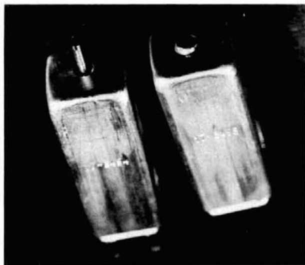
fig. 1. Two versions of the standard 1.9-cm (0.75-inch) i-f transformer, showing the different methods of tuning the inductor. (B) shows the connection pins at the base of the transformer.
