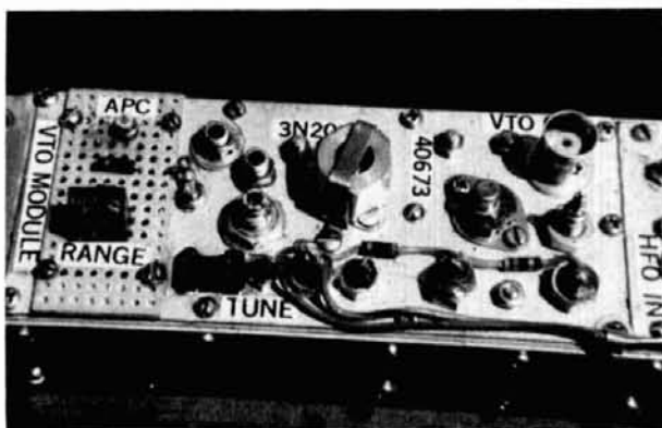
Since the VTO is dc tuned, it does not have to be located near the front panel. In this case, it has been incorporated into the same module as the HFO buffer.
